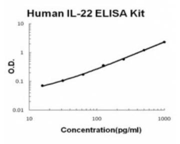
This standard curve was generated for demonstration purpose only (A standard curve must be run with each assay).
